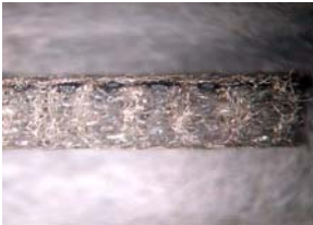
Fig 2 Cross Section showing Multi-planar fiber distribution (10X)
